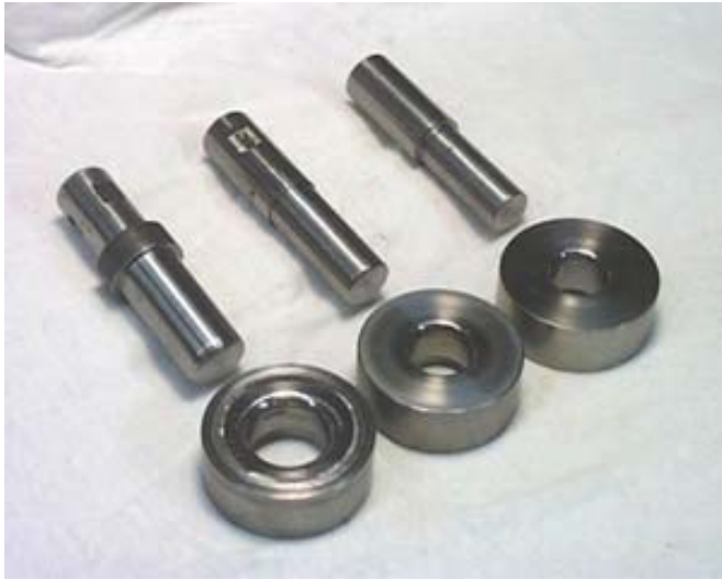
Drawing die and punch inserts used in my production die set.
