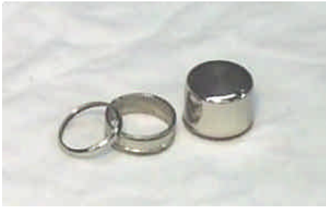
Cap & ring reel seat parts made from drawn cups
