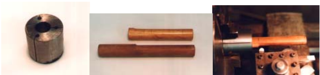
Photos: (l to r) Eccentric turning fixture; two insert blanks (one as turned, one finished); fixture in lathe with insert.
