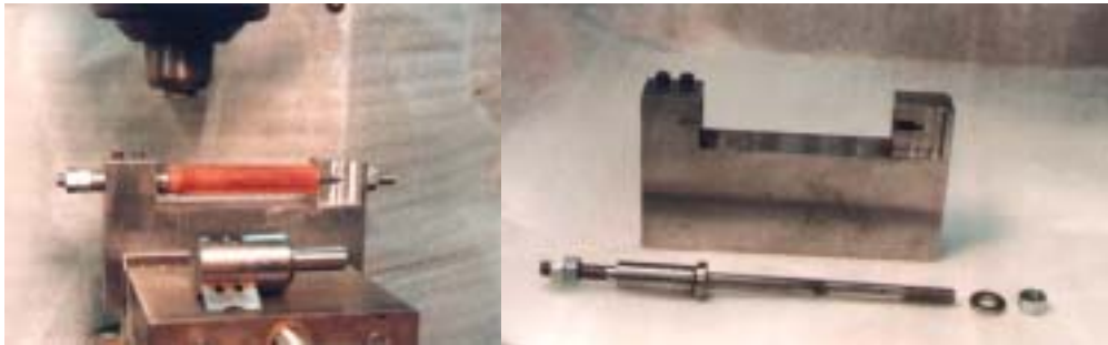
Photos: Fixture with blank in mill; fixture disassembled
